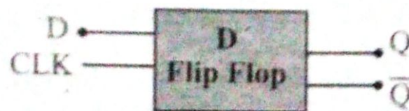
(Logic symbol for clocked D flip flop)
