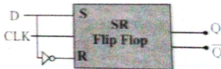
(SR flip flop converted into D flip flop)
